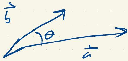
Properties:  $\vec{a} \times \vec{b}$  is perp to  $\vec{a}$ , perp to  $\vec{b}$
