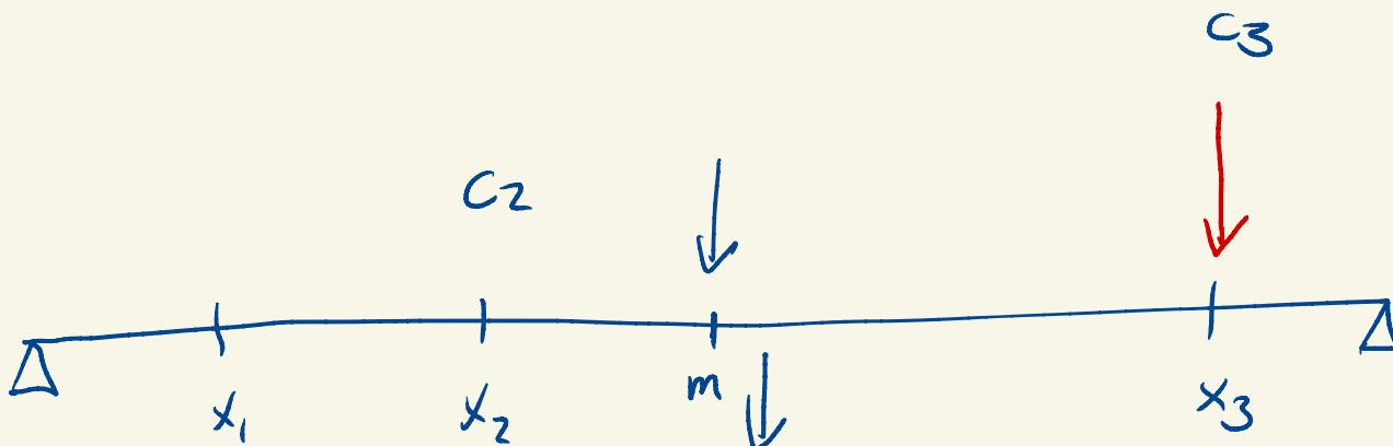
Want to measure the sag of the beam at  $m$
