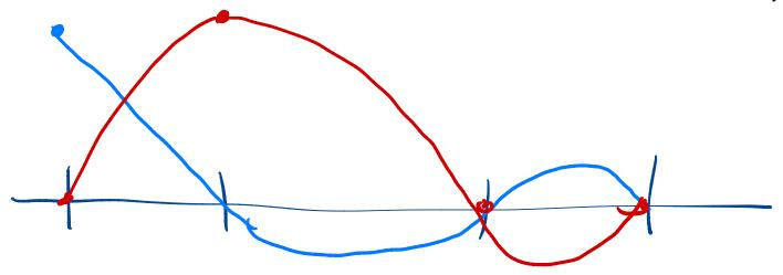
Strategy: We subdivide [a, b] into n equally sized intervals and interpolate with a polynomial of degree n. The case n = 1 is the trapezoid rule. The case n = 2 is known as Simpson's rule.
