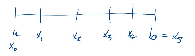
Strategy: We subdivide [a, b] into n equally sized intervals and interpolate with a polynomial of degree n. The case n = 1 is the trapezoid rule. The case n = 2 is known as Simpson's rule.
